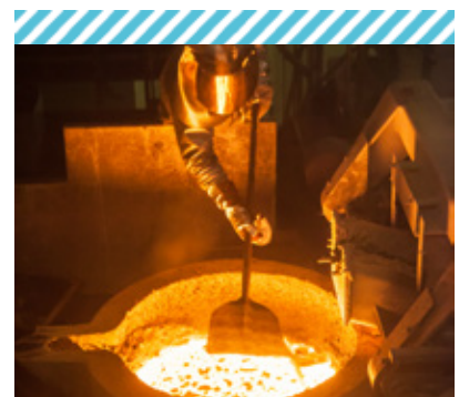
Operator working on the Centraco melting furnace
