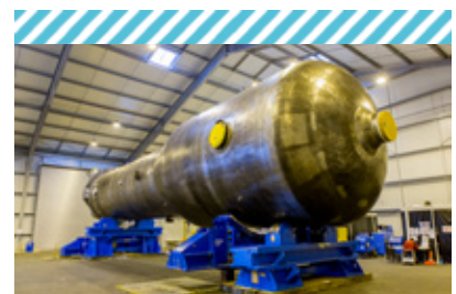
Steam generator for use in EDF's pressurised water reactors
